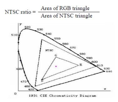
Note 8: Definition of optical measurement system.
